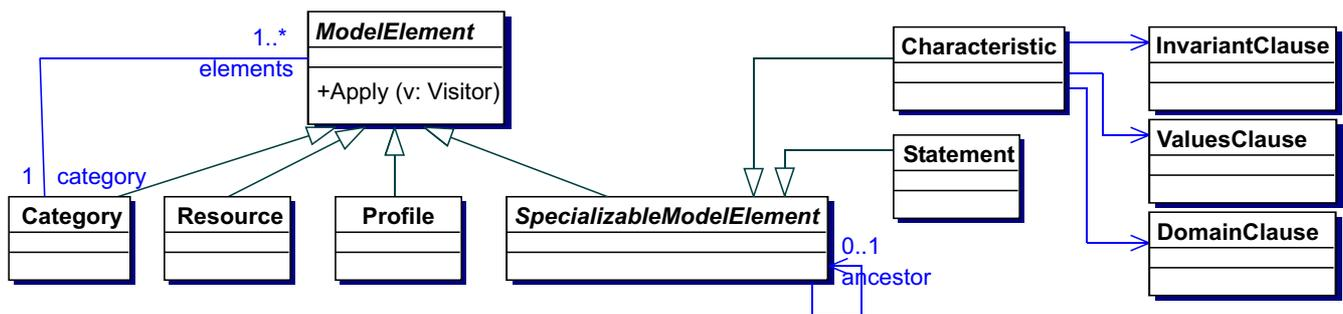
Fig. 10 Core classes of the CQML+ meta-model
