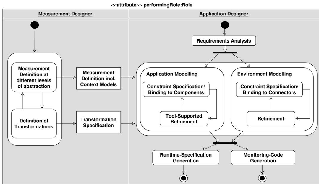
Fig. 1 Development process for non-functional properties overview
